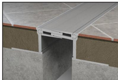
All metal seismic floor expansion joint for exterior and interior use, made of 2 aluminium side plates allowing expansion and contraction of the joint as well as vertical movement and shear movement.
